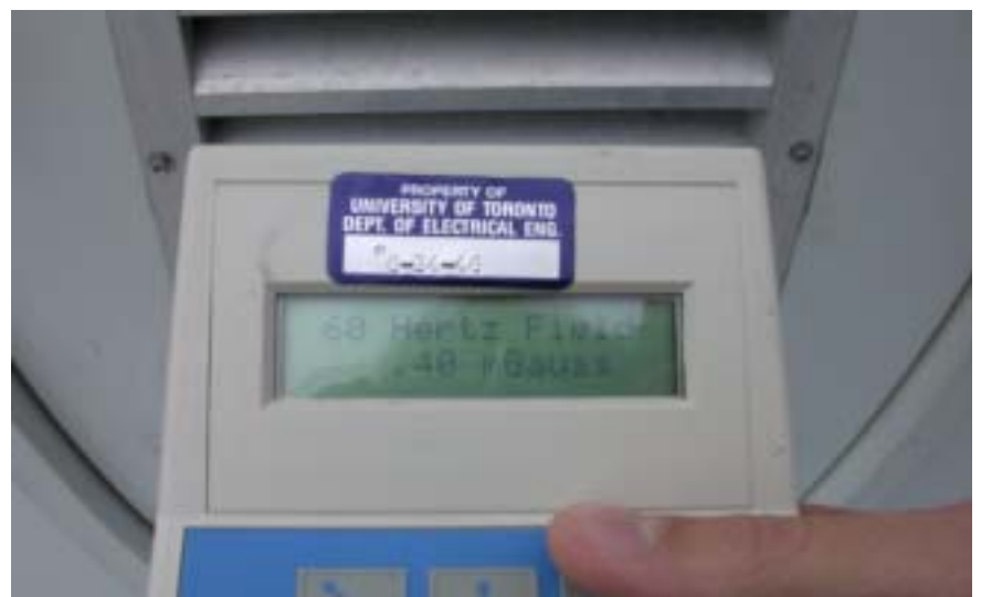
Measured in front door of the Windshare turbine installed at Toronto's CNE grounds = 0.4mG, one-half of a typical hair dryer with values of 0.8mG, compared to regulatory acceptable standard for emissions = 833mG.
